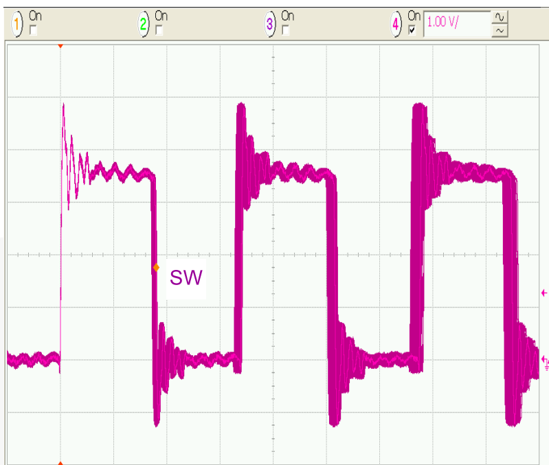
Figure 39. SW-Node Jitter (Infinite Persistence), I_{LOAD} = 200mA , 50ns/div.
