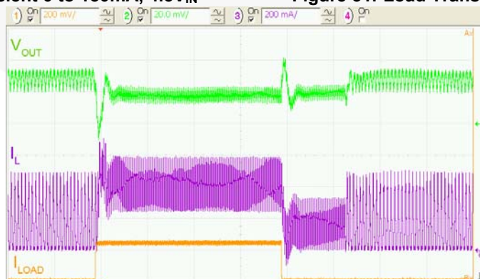
Figure 32. Load Transient 150 to 400mA, 4.5V_{IN}
