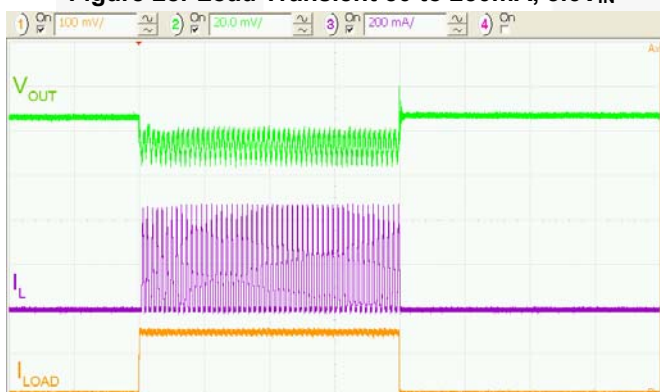
Figure 30. Load Transient 0 to 150mA, 4.5V_{IN}
