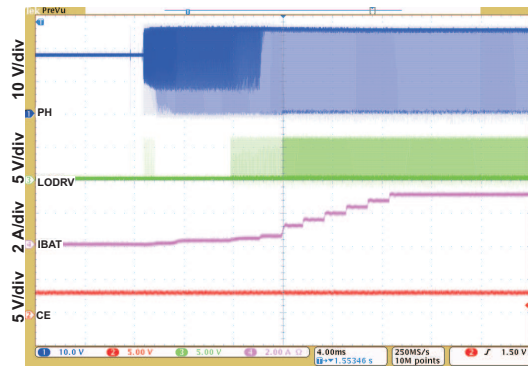
Figure 4. Current Soft-Start (CE = 1)
