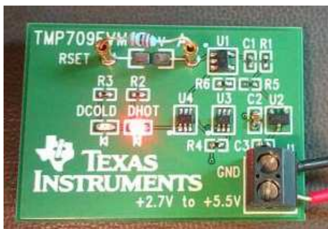
Figure 5. On-Board LEDs Indicating that Current Temperature is Above the Limit Set by Rset
