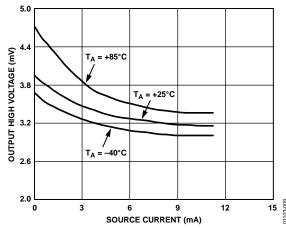
Figure 9. Output High Voltage, V<sub>OH</sub> vs. Source Current
