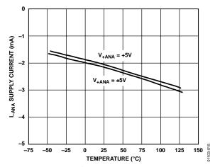
Figure 15. I<sub>-ANA</sub> Supply Current/Comparator vs. Temperature
