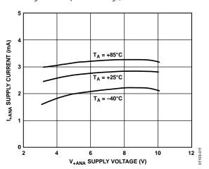
Figure 11. I<sub>+ANA</sub> Supply Current/Comparator vs. V<sub>+ANA</sub> Supply Voltage
