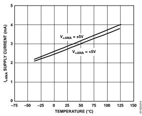
Figure 14. I<sub>+ANA</sub> Supply Current/Comparator vs. Temperature
