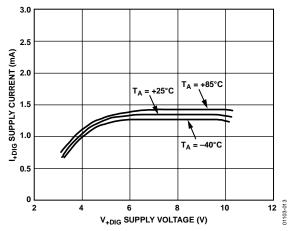
Figure 13. I<sub>+DIG</sub> Supply Current/Comparator vs. V<sub>+DIG</sub> Supply Voltage
