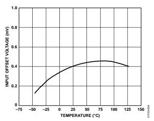
Figure 4. Input Offset Voltage vs. Temperature
