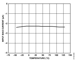
Figure 5. Input Bias Current vs. Temperature
