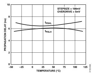
Figure 8. Propagation Delay, tpDHL/tpDLH vs. Temperature
