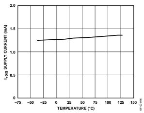
Figure 16. I<sub>+DIG</sub> Supply Current/Comparator vs. Temperature
