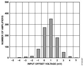
Figure 7. Input Offset Voltage Distribution
