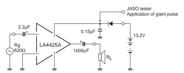
The over-voltage protector ( $V_{CC}X \approx 21.5V$ ) inside the IC is used to cut all bias routes and reverse bias between B-E of output stage elements, in order to increase the power line's capability of handling positive surge. This means, of course, that a  $V_{CES}$  ( $V_{CBO}$ ) type output stage element is used instead of the  $V_{CEO}$  ( $V_{CER}$ ) type.
