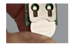
Note that when inserting the battery for the first time, the PCB contact point surface may have a thin layer of solder residue that can prevent contact with the battery. Remove and insert the battery a few times to power the SensorTag.
