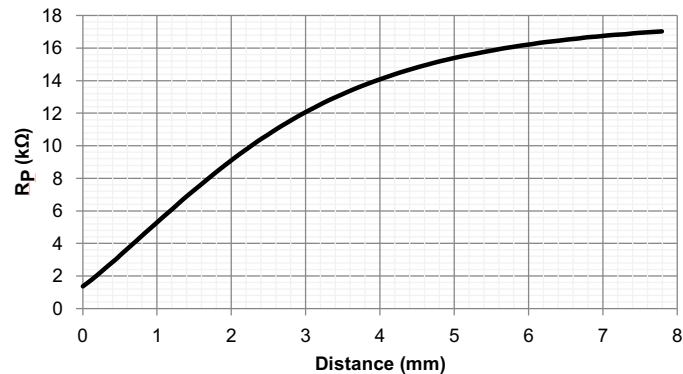
Figure 55. Example R_p vs. Distance with a 14-mm PCB Coil and 2mm Thick Stainless Steel Target
