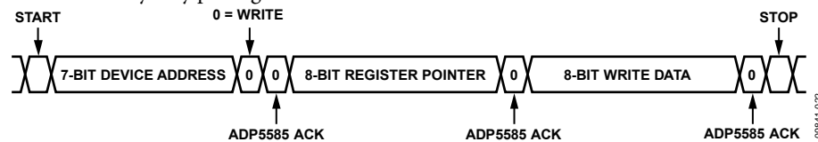
Figure 23. I 2 C Single Byte Write Sequence
