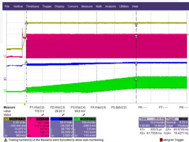
Figure 11. Soft-Start Characteristics, DC Mode, 200 V DC
