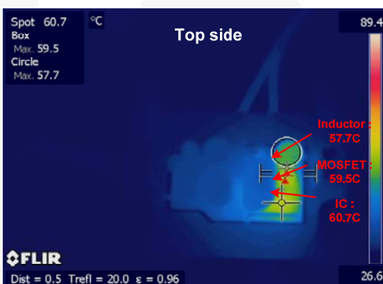
Figure 37. Thermal Test Result, Top-Side Temperature at 264 V AC Condition (Inductor)
