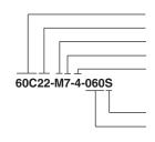
Angle of Throw: 22= 22.5° or 16 positions Rotation Torque: M= Medium torque
