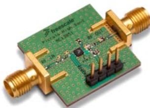
Figure 12. Typical Assembled Evaluation Board with SMA Connectors
