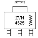
ZVN 4525 = Product Type Marking Code YWW = Date Code Marking Y or  $\overline{Y}$  = Last Digit of Year (ex: 5= 2015) WW or  $\overline{W}W$  = Week Code (01~53)
