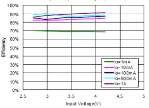
Efficiency vs Input Voltage (Vo=15V)
