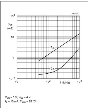
Fig.17 Input admittance as a function of frequency; typical values.
