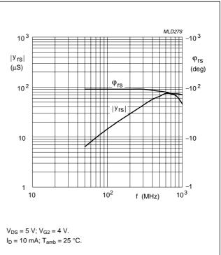
Fig.18 Reverse transfer admittance and phase as a function of frequency; typical values.
