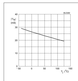
Fig.5 Transfer admittance as a function of the junction temperature; typical values.
