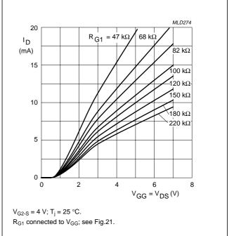
Fig.14 Drain current as a function of gate 1 (= V<sub>GG</sub>) and drain supply voltage; typical values.
