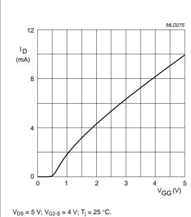
$V_{DS} = 5 \text{ V}$ ;  $V_{G2-S} = 4 \text{ V}$ ;  $T_j = 25 \text{ °C}$ .  $R_{G1} = 120 \text{ k}\Omega$  (connected to  $V_{GG}$ ); see Fig.21.
