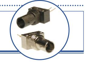
The OPF692 and OPF693 fiber optic transmitters are high performance devices packaged for data communication links. These transmitters are an 850nm GaAlAs LED and are specifically designed to efficiently launch optical power into fibers ranging in size from 50/125µm up to 200/300µm diameter fiber. Multiple power ranges with upper and lower limits are offered which allows the designer to select a device best suited for the application.
