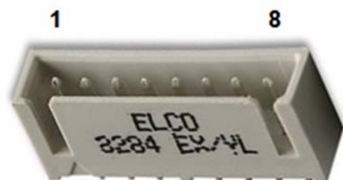
Figure 5. Analog Power Connector Pin Locations
