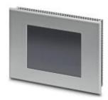
Touch panel with 14.5 cm/5.7" C-STN-Display (Resistive industrial touch screen), 320 x 240 Pixel (QVGA), 125 colors, ARM9<sup>™</sup>, 200 MHz, 2x USB Host 2.0, 1 x Ethernet (10/100 Mbps), RJ45, Windows CE 5.0 and User software: Visu+ / AX OPC Server. (Bus system: without)
