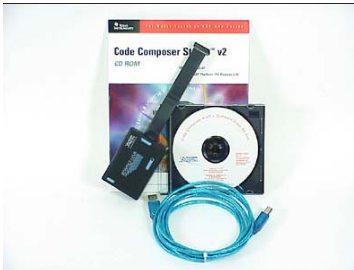
XDS510 USB JTAG Emulator with Code Composer Studio C2000 version 3.3
