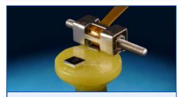
**SQUIGGLE RV motor and driver –** all kits integrate an SQL-RV-1.8 SQUIGGLE RV motor and NSD-2101 drive ASIC into a mechanical and electrical reference design.
