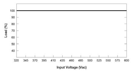
No output power de-rating across the entire input voltage range 3 x 320-600Vac (3-Phase) or 2 x 360-600Vac (2-Phase)
