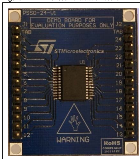
Figure 1. VND5E050K evaluation board
