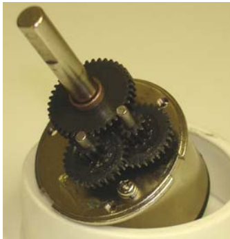
Spur-gear motor internals
