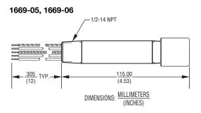
The 'single ended' protectors are useful for field devices with dual conduit ports; the field wiring connects to one port while the 1669 protector connects into the second - all connections are made within the instrument's wiring cavity. This installation simplifies the task of maintenance or of adding a protector into an existing loop.
