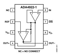
Figure 4. Pin Configuration
