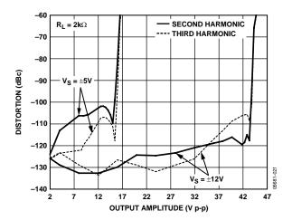
Figure 18. Harmonic Distortion vs. Output Amplitude and Supply Voltage (f=10 kHz)
