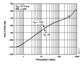
Figure 13. Isolation vs. Frequency—Disabled
