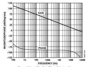
Figure 47. Amplifier Gain/Phase Relationship
