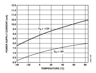
Figure 34. Power Supply Current vs. Temperature
