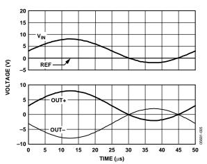
Figure 44. Typical Input/Output Response—Unequal Input/Reference
