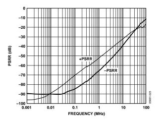
Figure 19. PSRR vs. Frequency
