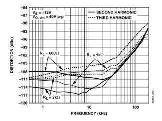
Figure 20. Harmonic Distortion for Various Loads
