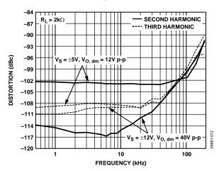
Figure 2. Harmonic Distortion for Various Power Supplies
