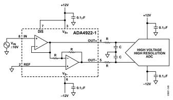
Figure 50. Driving a Differential Input ADC
