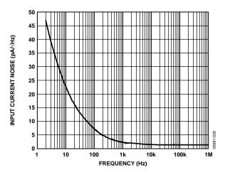
Figure 25. Input Current Noise vs. Frequency
