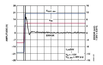
Figure 31. Settling Time,  $V_S = \pm 12 V$
