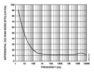
Figure 22. Differential Output Noise vs. Frequency
