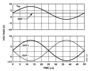
Figure 43. Typical Input/Output Response—Equal Input/Reference
