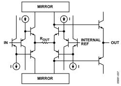
Figure 46. Output Stage Architecture
