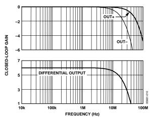
Figure 48. Closed-Loop AC Gain (Differential Outputs)
