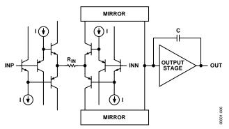
Figure 45. Internal Amplifier Architecture
