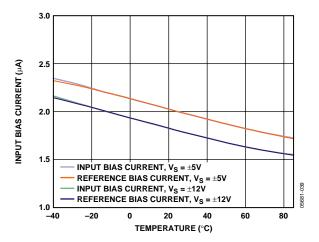
Figure 35. Input Bias Current vs. Temperature
