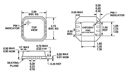
Figure 52. 8-Lead Lead Frame Chip Scale Package [LFCSP\_VD] 3 mm × 3 mm Body, Very Thin, Dual Lead (CP-8-2) Dimensions shown in millimeters
