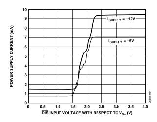
Figure 37. Power Supply Current vs. Disable Input Voltage
