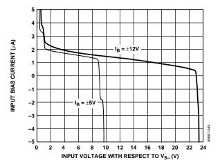
Figure 38. Input Bias Current vs. Input Voltage
