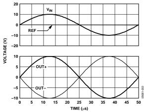
Figure 42. Typical Input/Output Response—Centered Reference
