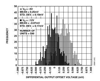
Figure 33. Differential Output Offset Voltage Distribution
