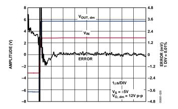
Figure 28. Settling Time,  $V_S = \pm 5 V$
