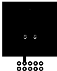
a) 55^\circ\text{C}/\text{W} when mounted on a 1\ \text{in}^2 pad of 2 oz copper
