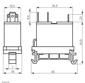
**Product code structure** 0430 2 5 09 100 Typical product code Type **0430** Power relay 430 3mm Mounting PCB version Snap mounting DIN-rail mounting Mounting brackets Contact design 4 Arc blowing magnet Standard Coil Coil code: please refer to coil versions table **Contact material** O AgCu 3 1 AgCdO Version 100 Standard
