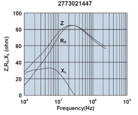
Impedance, reactance, and resistance vs. frequency.
