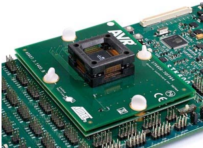
Figure 1-1. STK600 router and socket card
