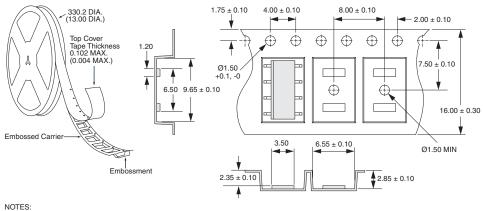
NOTES: 1. All dimensions in millimeters 2. 10 sprocket hole pitch cumulative tolerance ± 0.20. 3. Carrier camber is within 1mm in 250mm.
