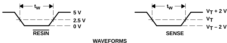
Figure 2. Input Pulse Definition
