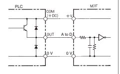
Note: 1. Use the M7F positive logic input model if the PLC Output Unit has PNP output.
