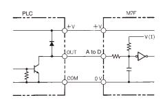
Note: The PLC connects to the M7F with ease via the G79-□C Cable (with connectors, sold separately).
