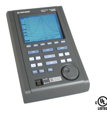
The 2650 and 2658 are high-performance handheld spectrum analyzers providing excellent performance and functions perfect for many different applications. It is a compact, lightweight and cost-effective unit that is ideal for testing W-CDMA, CDMA, GSM, PDC, PHS, Wireless LAN and Bluetooth systems.
