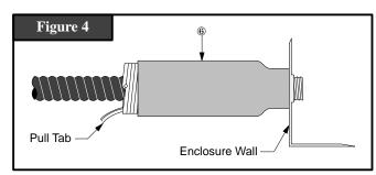
**5.** Position Cold Shrink Corrosion Protection Assembly ® (*Figure 4*) over bulkhead termination connector. Install by unwinding loose core pull tab in a counter-clockwise direction around cable. Rubber sleeve should make contact with enclosure wall during installation.
