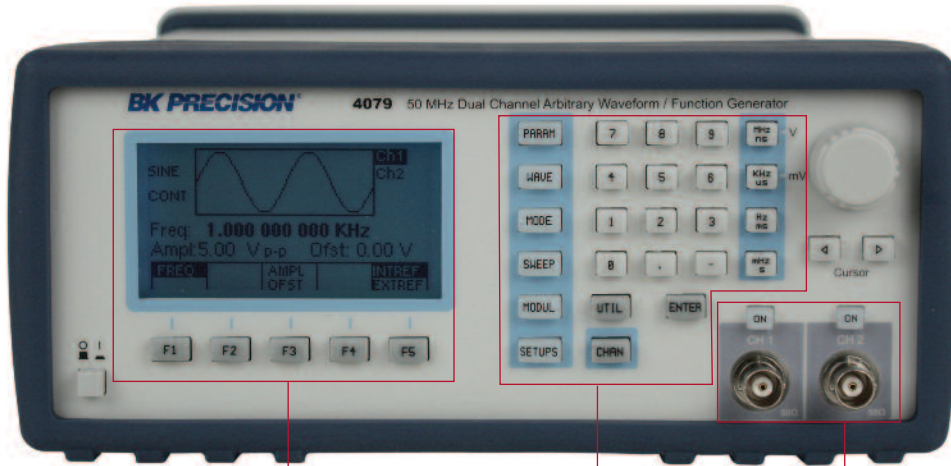
Informative LCD with detailed display of waveform parameters
