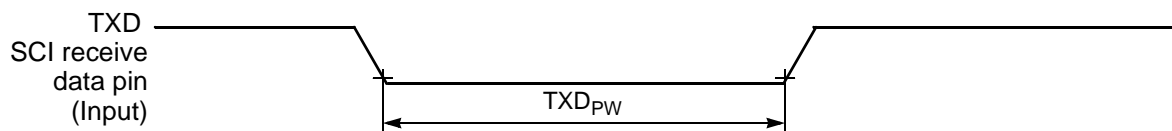
Figure 10-17 TXD Pulse Width
