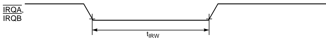
Figure 10-6 External Interrupt Timing (Negative Edge-Sensitive)
