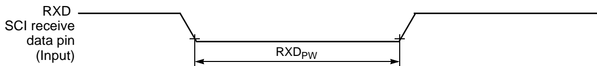
Figure 10-16 RXD Pulse Width
