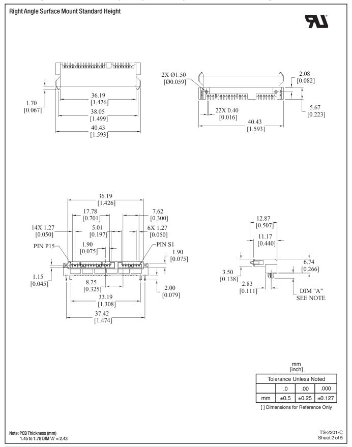
Host Receptacle, Vertical and Right Angle, Std Height, Surface Mount Receptacle
