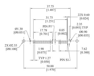
RECOMMENDED PCB LAYOUT TOLERANCE:  $\pm 0.05 [0.002]$
