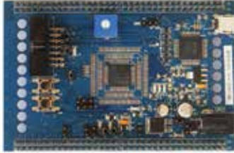
SPC56D-Discovery with SPC560D40L1 order code: SPC560D-DIS
