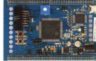
SPC56B-Discovery with SPC560B54L5 order code: SPC560B-DIS
