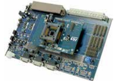
SPC56 Mother Board with mini-module Order code: see Board Summary table
