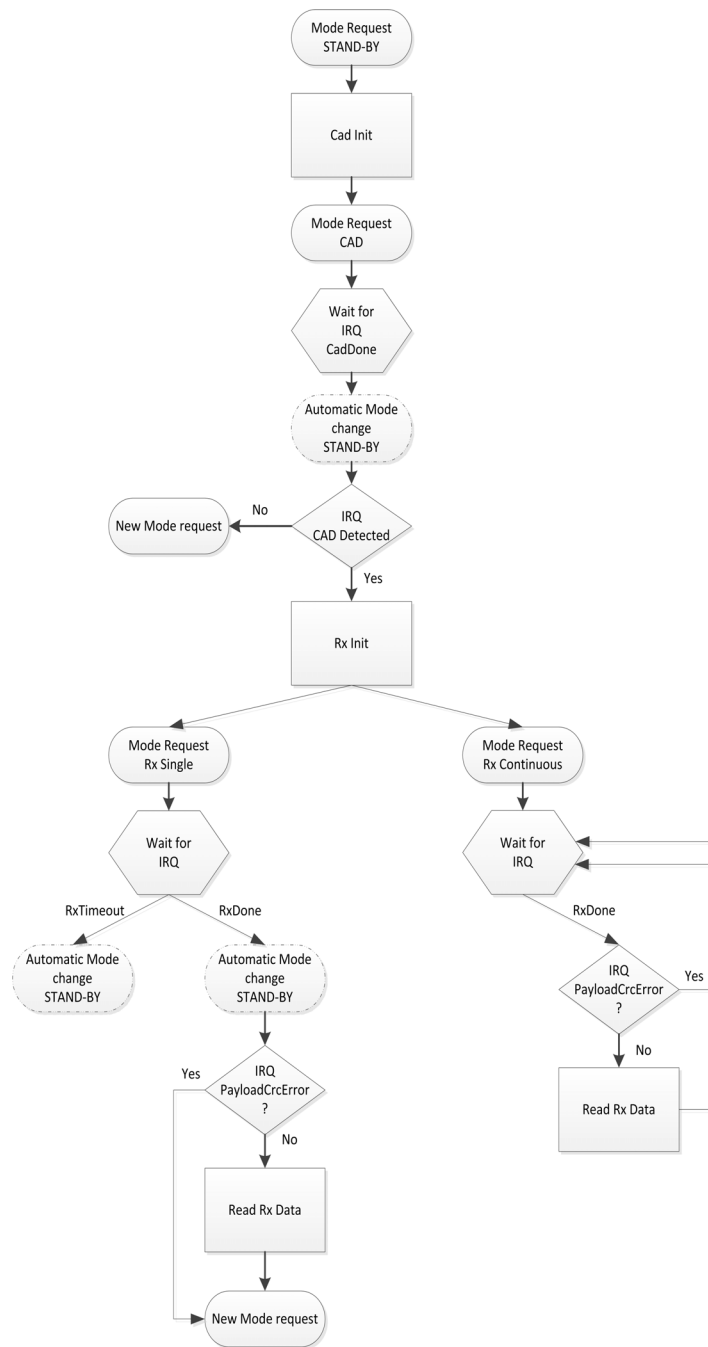
Figure 12. LoRa™ CAD flow
