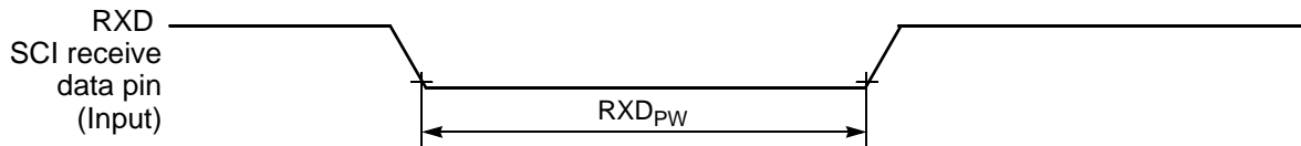
Figure 3-25 RXD Pulse Width
