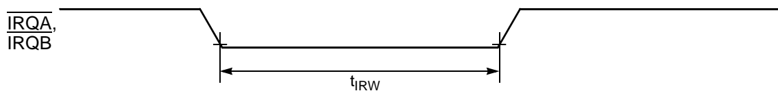
Figure 3-13 External Interrupt Timing (Negative-Edge-Sensitive)
