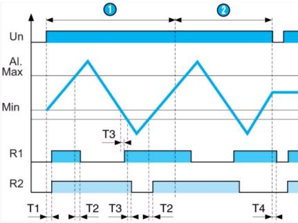
On power-up, probe AI. is submerged, relays R1 and R2 are energised and the pump is ON: filling starts, the LED for relay R1 is lit. When the level reaches the Max probe, relay R1 de-energises and the pump is OFF: filling stops, the LED for relay R1 goes off. Relay R1 re-energises when the Min probe emerges. In the event of a fault (level continues to fall) probe AI. emerges, relay R2 deenergises ans the alarme is triggered: the LED for relay R2 is lit.
