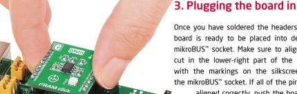
Once you have soldered the headers your board is ready to be placed into desired mikroBUS™ socket. Make sure to align the cut in the lower-right part of the board with the markings on the silkscreen of the mikroBUS<sup>™</sup> socket. If all of the pins are aligned correctly, push the board all
