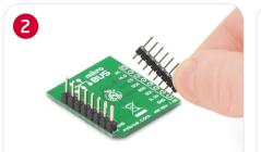
Turn the board upside down so that bottom side is facing you upwards. Place shorter parts of the header pins in both soldering pad locations.
