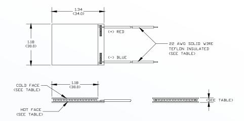
Ceramic Material 96% Alumina Ceramics Solder Construction: 138°C BiSn
