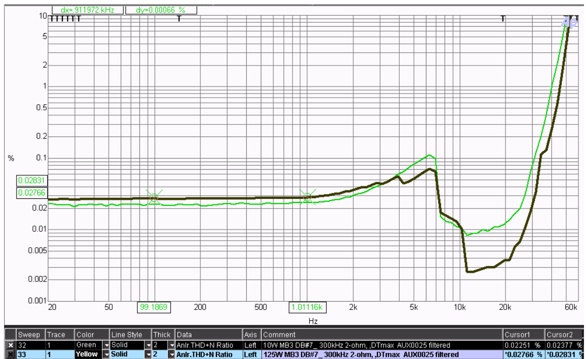
Figure 4 THD+N vs. Frequency at 10W and 125W
