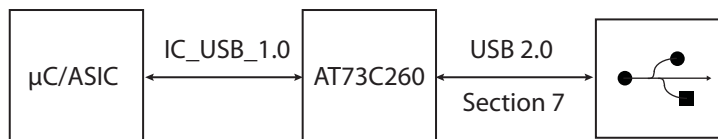
Figure 9-20. ICC_S7 Block Diagram
