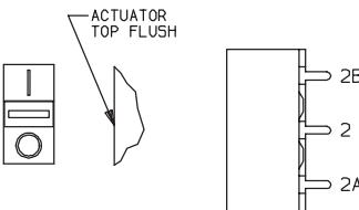
Markings are reversed on V702 and V802 models. **Note:** Orientation of actuator markings and terminals.
