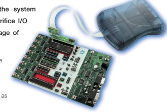
The JTAGICE mkll interface is integrated in AVR Studio, Atmel's front-end tool for development on the AVR architecture. All phases of the AVR development can be done in this Integrated Development Environment.
