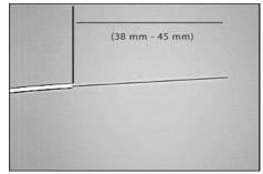
Note: Do not wipe the fibers more than two times, and limit the time that the bare fiber is exposed to the atmosphere.
