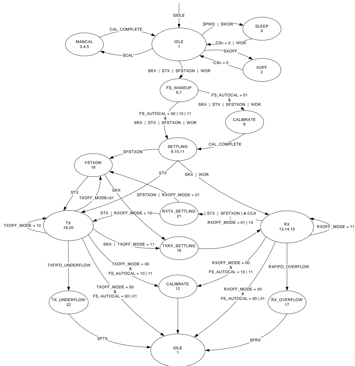
Figure 20: Complete Radio Control State Diagram
