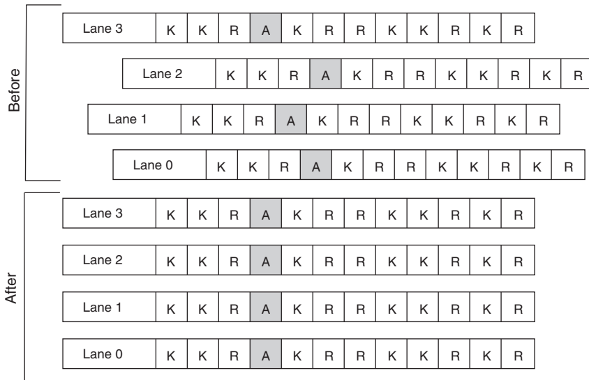
Figure 2–19. Before and After the Channel Aligner
