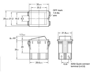
Note: Unless otherwise specified, a tolerance of  $\pm 0.4$  mm applies to all dimensions.
